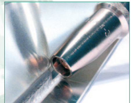
MIG - flat-wire welding of aluminium, welding speed: 2 m/min.
